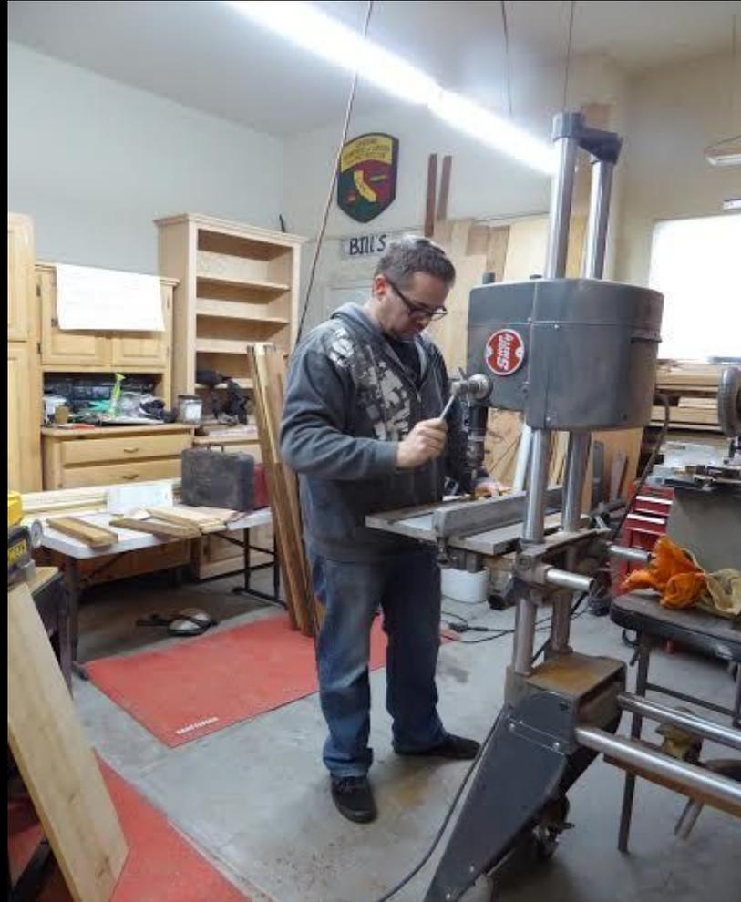
Three holes were drilled on each board. one for each peg.
