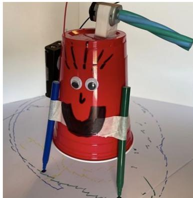
11. What modifications can you make to change the movement of the vibrobot by adjusting the position of the eraser, the markers, the battery pack, and the motor.
