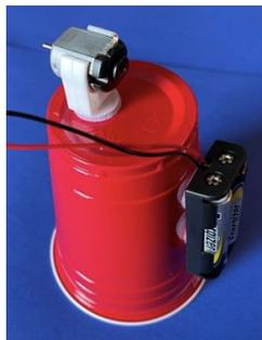
5. Attach the positive wire to one copper mount on the motor. Attach the second wire when you have completed your robot and are ready to make it move. You can test the two wires touching the copper mount on the DC motor, but then remove one wire to finish building your artbot.
