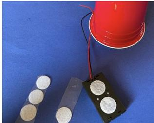
3. Attach the battery pack to the side of the cup with the positive (red) and negative (black) wires pointing up. Gently bend the exposed wire on the positive and negative leads so that they can hook to the DC motor copper connection.
